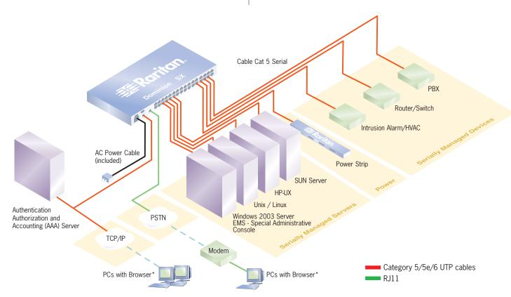
**NOTE:** On certain servers, depending on serial pin-outs, an adapter may be required \***Remote User** - Administration of Dominion SX <u>and</u> access to serially managed servers and other devices
